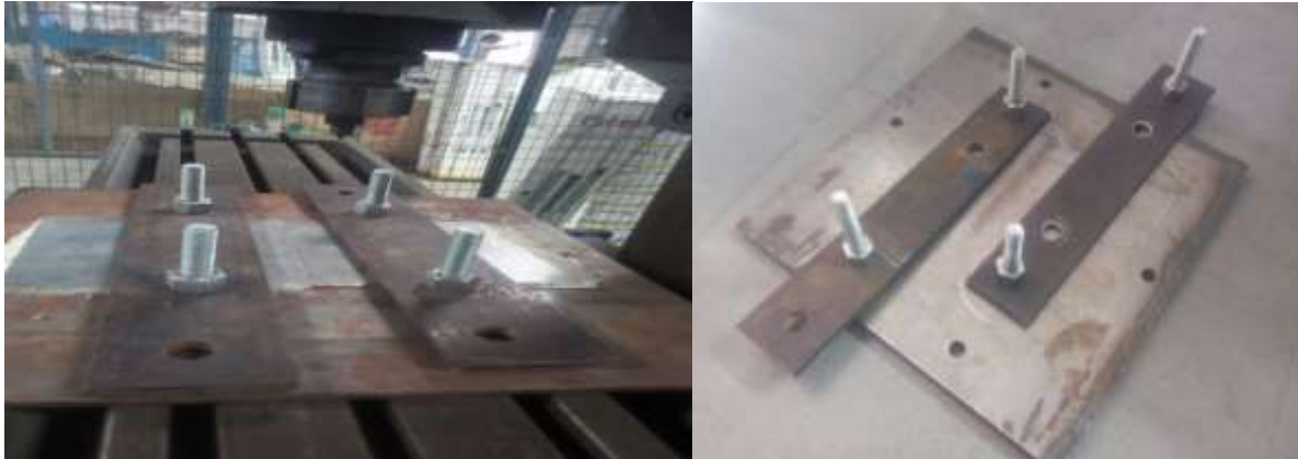
Figure 2 Setup and clamping of FSW plates
